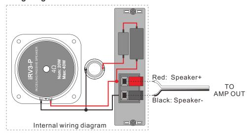
**Attention:** When connecting the output lines of the power amplifier, the positive and negative stages of the speakers on the two wiring card holders should not be connected incorrectly, as incorrect connections can cause poor sound.
